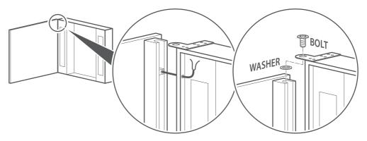
Attach the door at the top and bottom using the bolts and washers provided.
