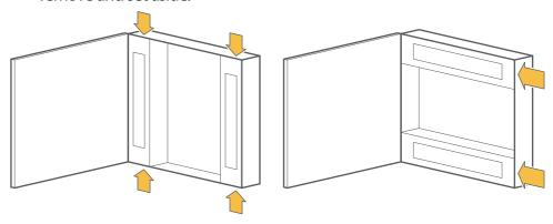
Carefully align and push the door demister cable through the gap in the side of the cabinet **a**) until the door is fully positioned under the hinge plate **b**).
