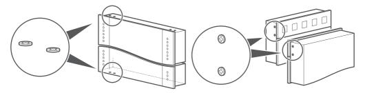
Carefully push the door demister cable through the grey grommet. The entry position will depend on the model.
