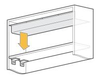
Feed the door demister cable through the grey grommet located on the electrics cover.
