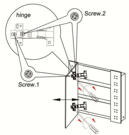
• Mirror door will be moved inwards or outwards from the cabinet by adjusting **Screw.2** towards the left-hand side or right-hand side respectively, as shown below.
