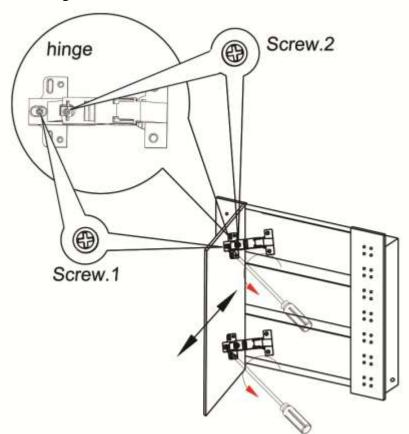
• After loosening **Screw.1**, please move the mirror door to the left or to the right, and make sure the mirror door is in the middle between two side mirror panels as show in the below diagram.
